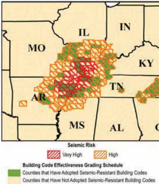
Figure 10. Map showing counties in NMSZ that have high seismic risk, relative to their building code adoption for commercial buildings (FEMA).
