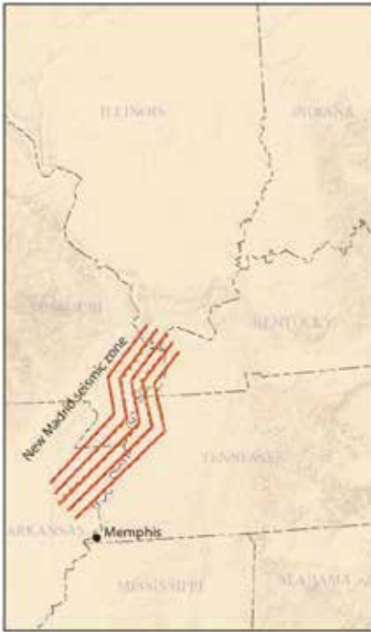
Figure 8. Representation of the five fault traces of NMSZ (2014 USGS Report).
