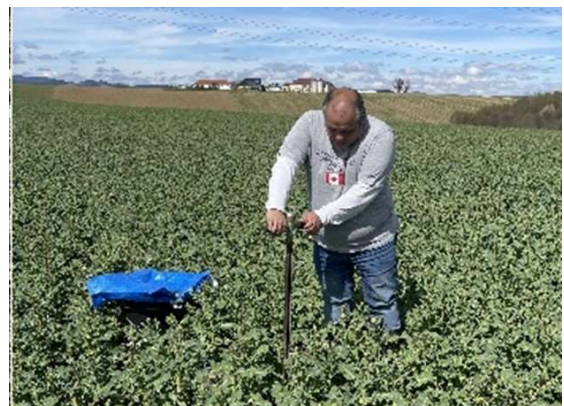
Figure 2. Soil sampling and natural gamma-radiation ( ^{40}\text{K} , ^{238}\text{U} , and ^{232}\text{Th} ) measurement using mobile Gamma-ray sensor. model MS 350 in Petzenkirchen, Austria.
