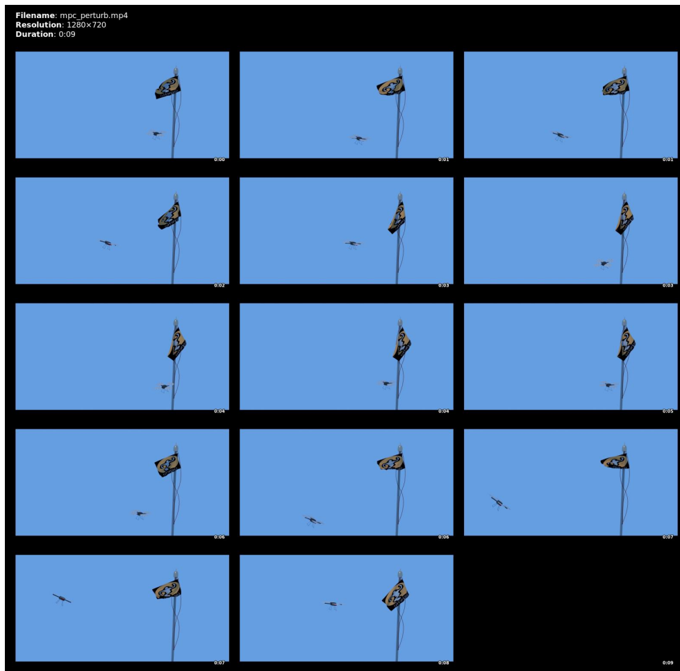
Figure 2.9: Video screen shots: MPC with the quadrotor – wind perturbation.
