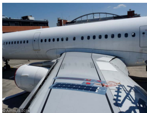
Figure 8: A321 left wing implementation of the wireless sensors together with the battery-free power supply based on solar energy harvesting and storage on supercapacitors.
