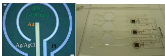
Figure 13: (Au - Pt - Ag/AgCl) ElecCell technological platform (left) and ElecCell integration on transparent glass substrate for algae cultures monitoring (right)
