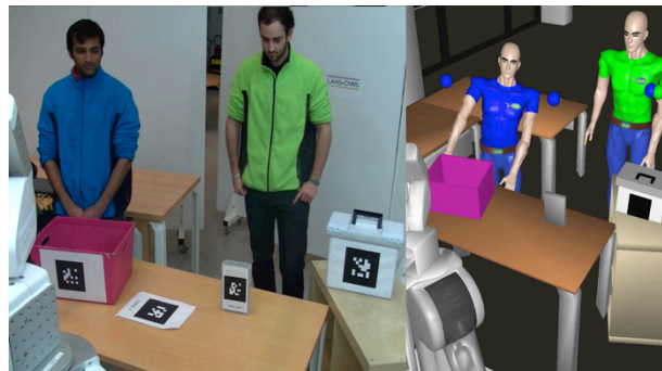
Figure 16: A Collaborative Robot Able to Estimate its Partners Perspective View of the Situation
