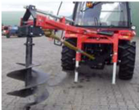
Fig. 1 - Drilling machine for drilling holes mounted on tractor[13] Fig.2 - Drilling pits equipment [13]
