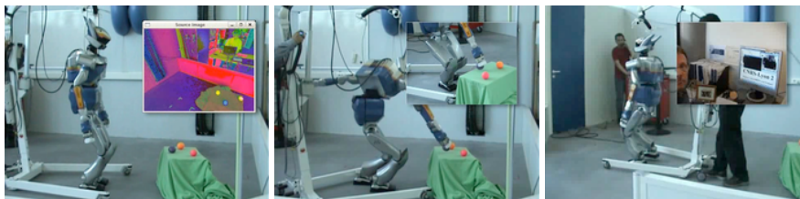
Figure 5.11: Teleoperated by an operator located in Lyon through natural language interaction, the HRP-2 robot in Toulouse looks for a ball with its vision system and grasps it autonomously
