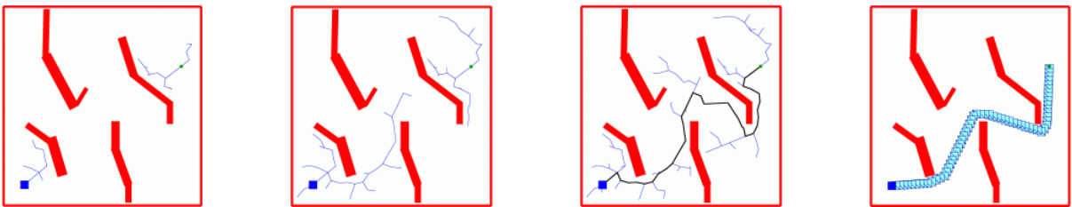
Figure 5.2: The sequence of images shows snapshots of two RRTs during the planning process for a simple 2D example. The final image shows the computed path after optimization.
