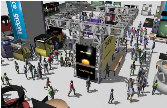
Figure 1: Navigation within an indoor environment: An exhibit hall of a trade show that consists of 511 booths and 1,000 human agents. Each agent has a distinct goal (i.e. visiting one of the booths) and behavior characteristic. Our navigation algorithm based on AERO can compute collision-free paths simultaneously for all 1,000 agents at 22 fps on a PC with 3Ghz Pentium D CPU.
