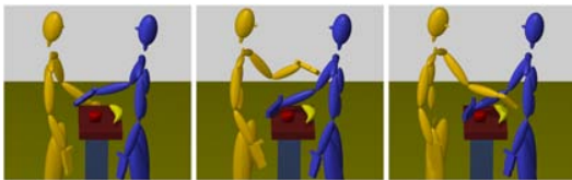
Figure 3: The motion of the character on the left side was planned after the motion of the character on the right side, achieving synchronized simultaneous grasping.
