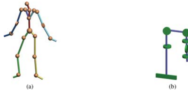
Fig. 2. Our virtual characters are represented as tree-like structures formed of rigid bodies linked with spherical, rotational, and planar joints.
