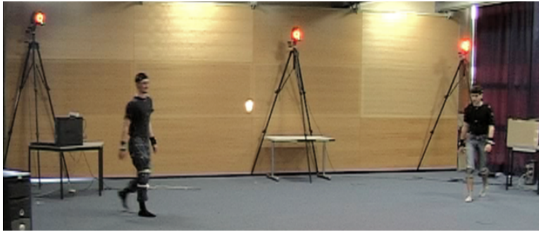
Figure 5.6: Using a motion capture system, we recorded and analyzed hundreds of pairs of participants having interacting trajectories. A well-defined protocol allowed us to understand some key factors during reactive navigation tasks executed by Humans.
